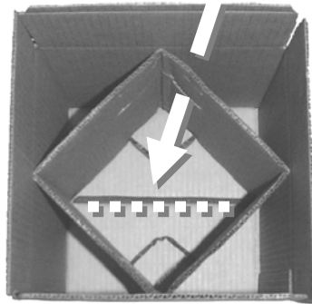
Bottom flap forms "ridge" in outer box
